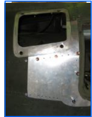
New repaired skin on TR's turtle back, thanks o Scott Hochstein. Photo by Col K. Hong
