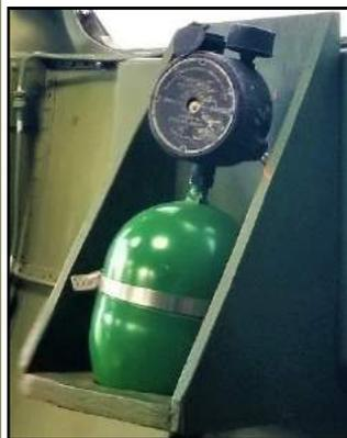
Combat damage sustained to either an oxygen bottle or an O2 line resulted in the automatic closing of one or more "check valves" located at each bottle and distribution points throughout the system.
