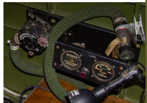
Figure: Radio Room Oxygen Station with A-12 Regular, pressure gauge, flow gauge & Warning light.
